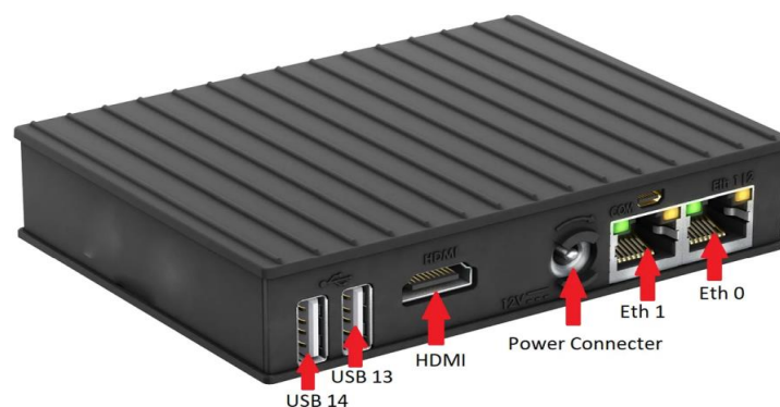
Figure 2: Horizon Power’s SGD hardware and port overview 1
