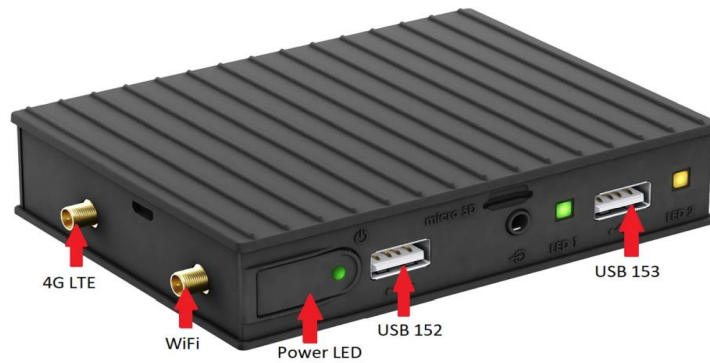
Figure 3: Horizon Power's SGD hardware and port overview 2
