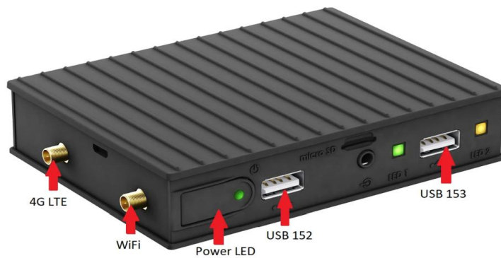
Figure 10: Horizon Power's SGD hardware and port overview 2
