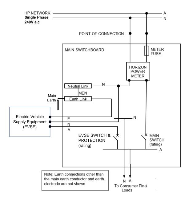
Note: For indicative purposes only. Contractors shall provide a single line drawing specific to the proposed installation. For more information refer to the Electric Vehicle Supply Equipment Technical Requirements available at:
